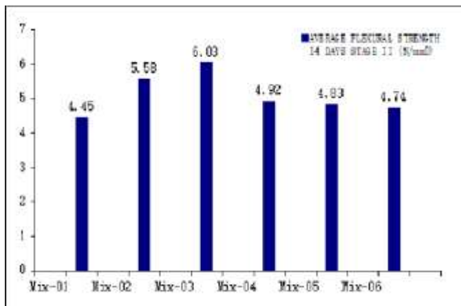
Figure 6. Flexural Strength in N/mm 2 at 14 days
